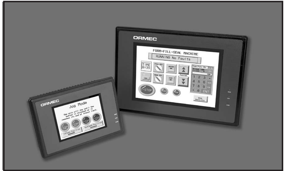
ORMEC's touchscreen operator interfaces provide a fully graphical, easy to use human-machine interface.
