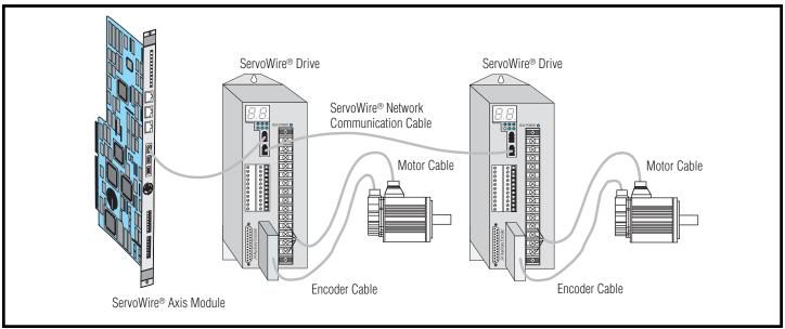
ServoWire® cable interconnection diagram for G-series servomotors.
