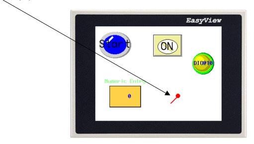
If a meter scale is desired it must be placed on the screen separately by clicking the **Scale icon** on the toolbar or from the **Draw** pull down list.
