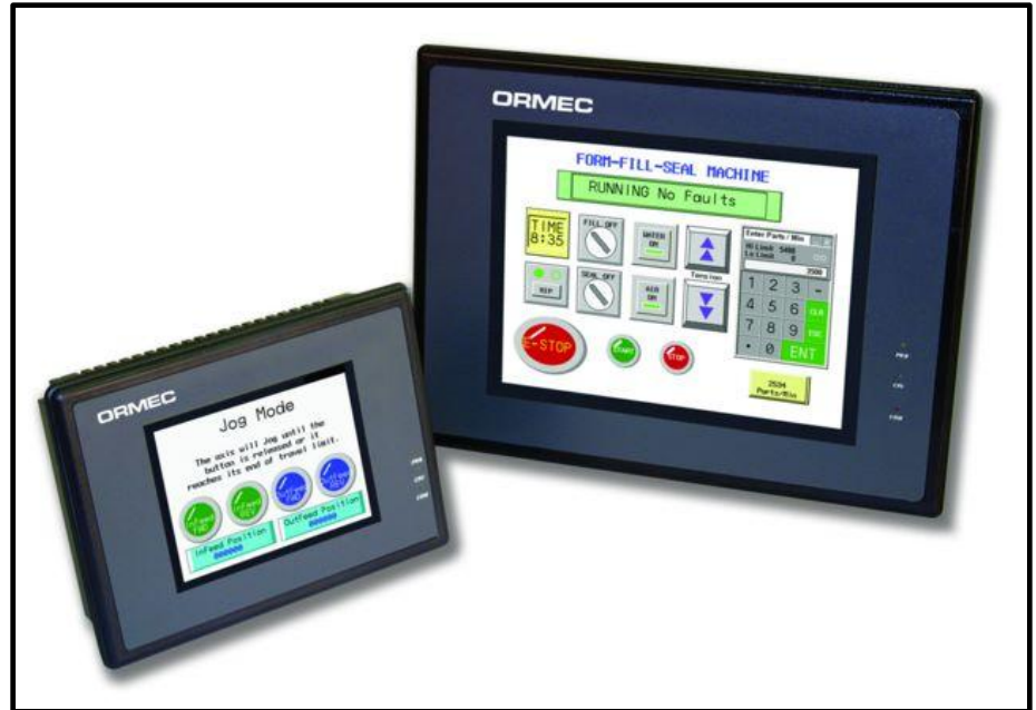
ORMEC's touch screen operator interfaces provide a fully graphical, easy-to-use human-machine interface.
