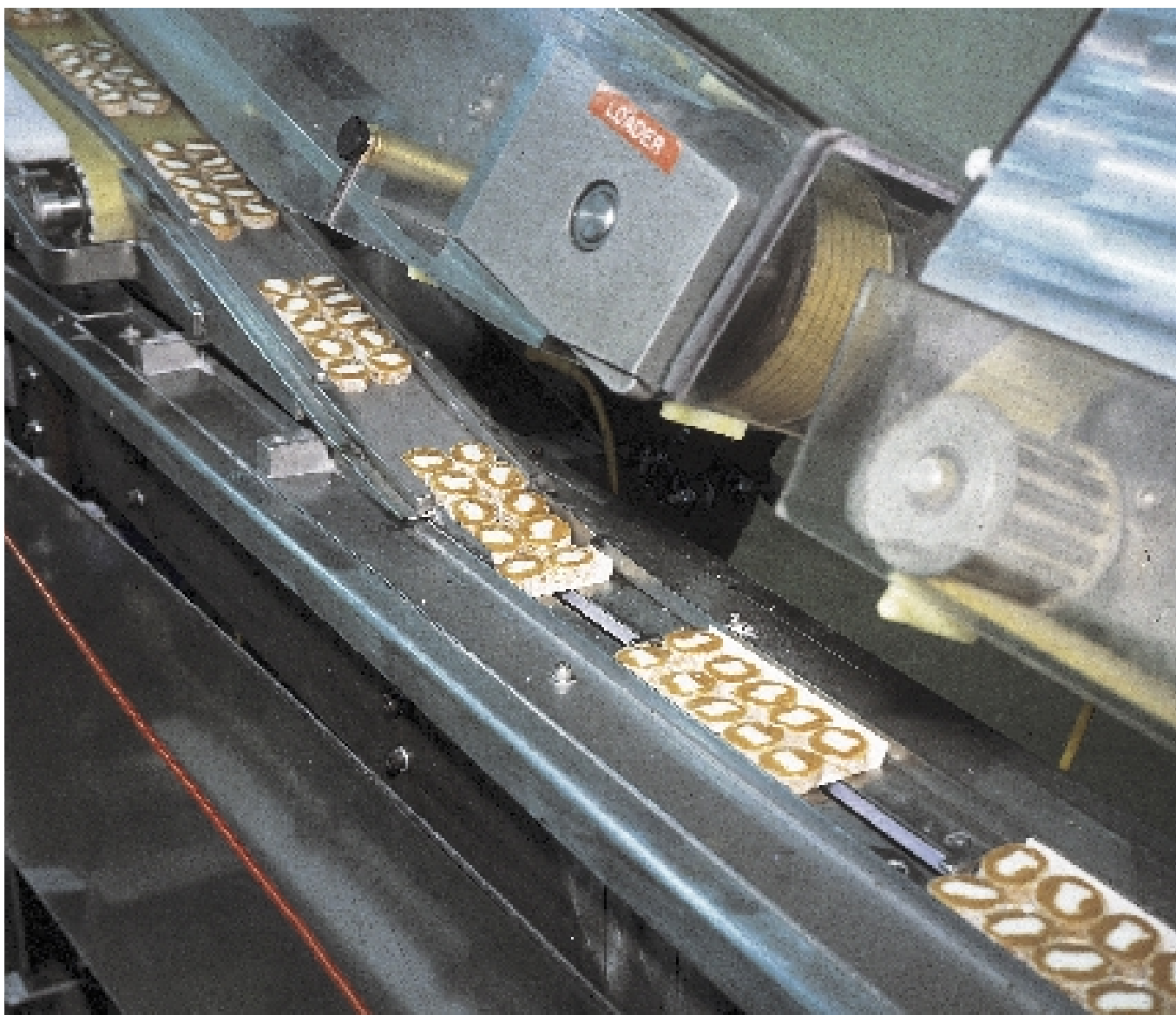
Candy groupings with missing pieces are automatically rejected from the belt by a rotating paddle arm (below). Next, candies are precisely positioned onto U-boards (above). Operators can adjust the timing of any motor right from the operator interface (bottom).
