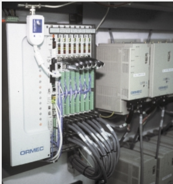
The motion controller (above) is actually a PC with seven dedicated plug-in cards for high-speed control.
