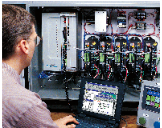
The screen machine motion controller provides interfaces to users, programmers, and upper-level management systems.
