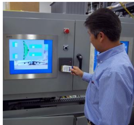
System includes a badge reader for secure system access.
