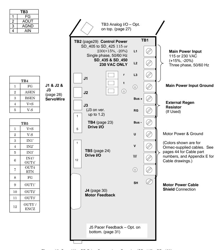
**Figure 12**, ServoWire SD Drive Connections Overview(SD\_417 – SD\_450)
