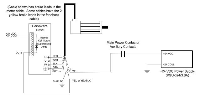
Figure 27, Fail-Safe Brake Interlock Circuit – SAC-SDx-R versions and –S versions 1.2 and later
