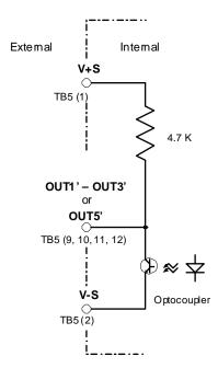
**Figure 19**, Schematic of Discrete Outputs OUT1'-OUT5', -S version, prior to version 1.2
