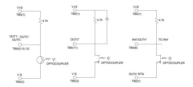
**Figure 20**, Schematic of Discrete Outputs OUT1'-OUT5', -R version and -S version 1.2 or later
