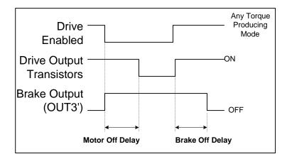
Figure 28, Brake Output Sequence of Operation
