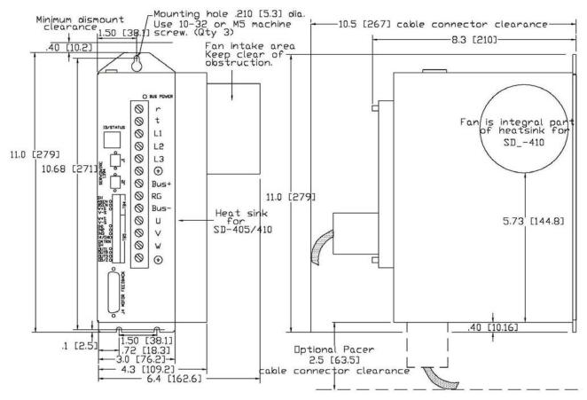
Figure 6, ServoWire SD Drives 405 & 410 w/ 1394 locking connectors, Outline Drawings
