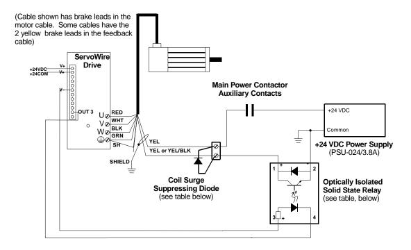
Figure 26, Fail-Safe Brake Interlock Circuit – SAC-SDx-S versions, versions before 1.2
