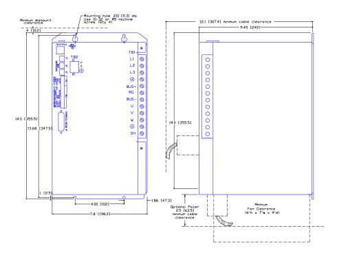
Figure 7, ServoWire SD Drives 435 & 460 w/o locking connectors Outline Drawings
