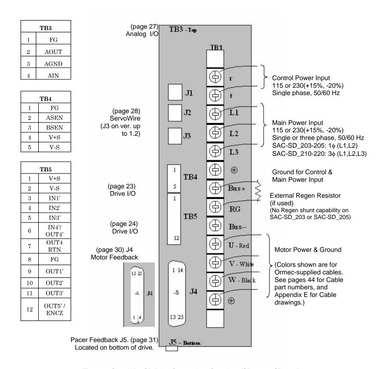
Figure 9, ServoWire SD Drive Connections Overview (SD\_203 - SD\_220)
