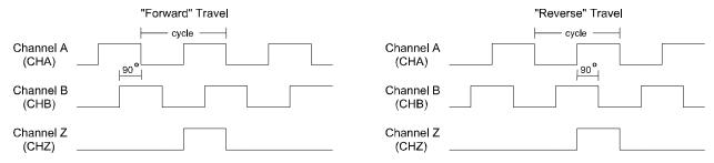
NOTE: Channel Z (once per revolution marker channel) is synchronized with Channel A.
