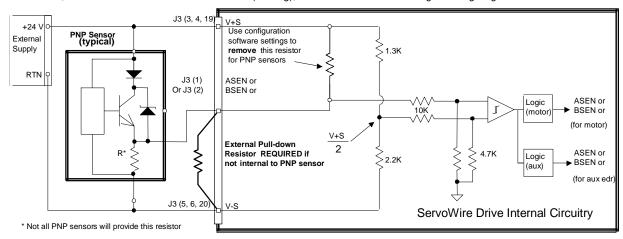
Figure 17, Schematic of ASEN and BSEN wiring for NPN and PNP sensors
