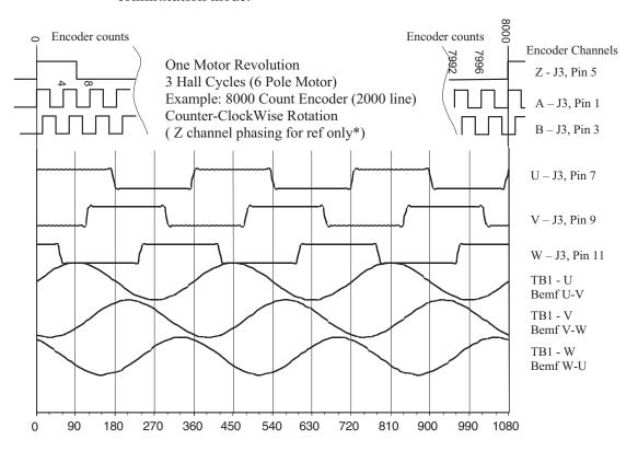
Figure 30, Hall signals and Motor Back EMF waveforms
