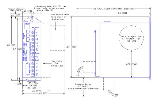
Figure 1, ServoWire SD Drives 203 - 220 Outline Drawings
