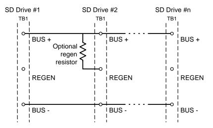
Figure 22, Bus Sharing Connections
