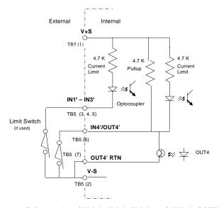
Figure 18, Schematic of IN1', IN2', IN3' and IN4'/OUT4' Inputs
