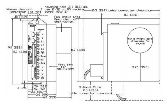
Figure 2, ServoWire SD Drives 203 - 220 with 1394 locking connectors, Outline Drawings
