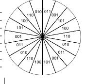
Figure 31, Valid Hall States (6 Pole Motor Example diagram)
