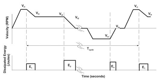
Figure 34, Regeneration during deceleration.
