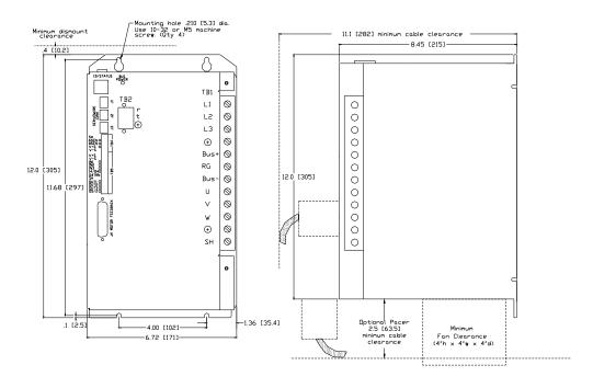
Figure 3, ServoWire SD Drives 225-260 & 417-425 w/o locking connectors, Outline Drawings
