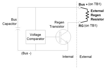
Figure 21, Regen Resistor Connection
