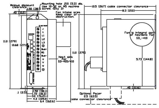
Figure 5, ServoWire SD Drives 405 & 410 w/o locking connectors, Outline Drawings
