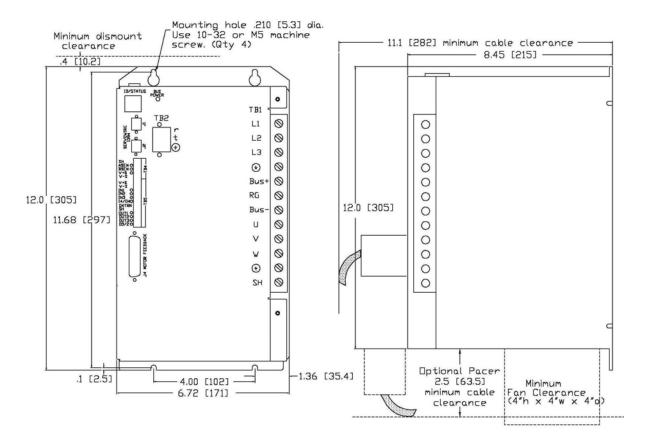
Figure 4, ServoWire SD Drives 225-260 & 417-425 with 1394 locking connectors, Outline Drawings
