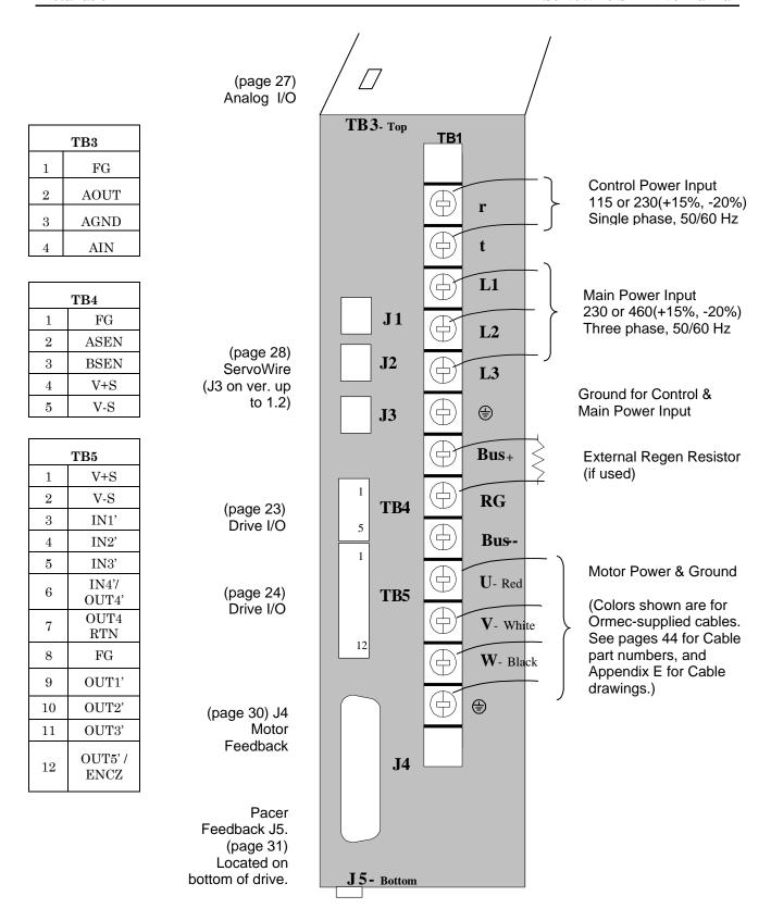
Figure 11, ServoWire SD Drive Connections Overview (SD\_405 – SD\_410)
