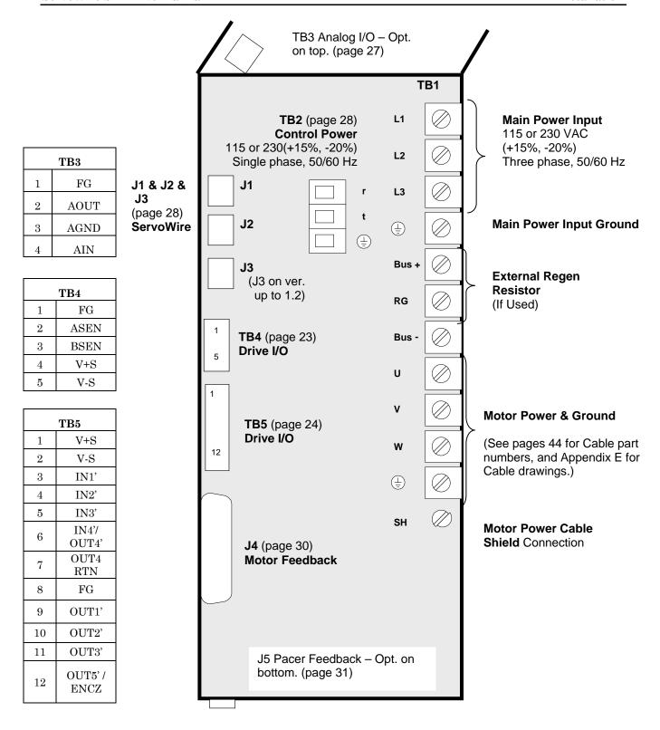
Figure 10, ServoWire SD Drive Connections Overview(SD\_225 - SD\_260)
