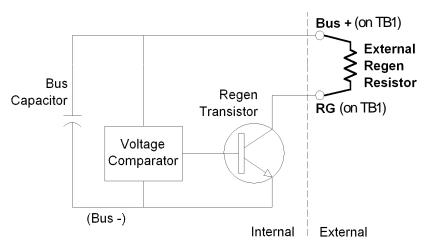
Figure 33, Simplified Schematic of Shunt Regulator
