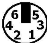
**Figure 12**, SMLC System Card - Keyboard Connector (J7) connector.
