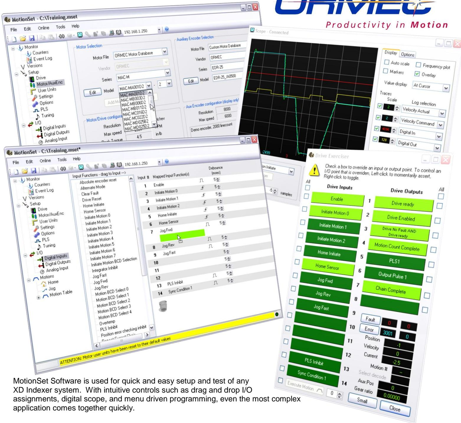
MotionSet Software is used for quick and easy setup and test of any XD Indexer system. With intuitive controls such as drag and drop I/O assignments, digital scope, and menu driven programming, even the most complex application comes together quickly.
