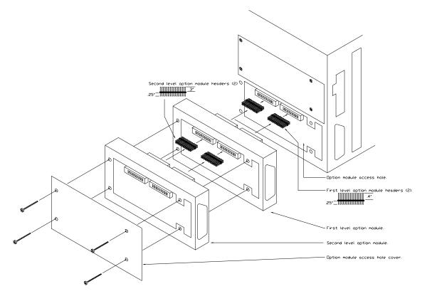
Figure 20, Feedback Option Module Installation 7
