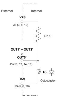
Figure 13, Schematic of Discrete Outputs OUT1'-OUT5'
