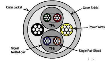
Figure 10, ServoWire Connector (J1 & J2) and Cable
