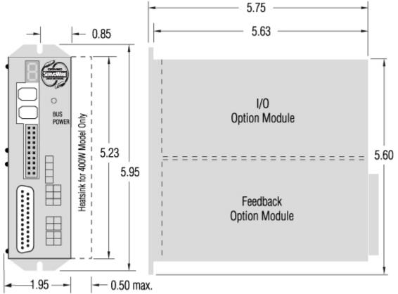
Additional clearance above, below and to the sides of the ServoWire Drives is also required for heat dissipation: SAC-SM\_A03 and SAC-SM\_A05
