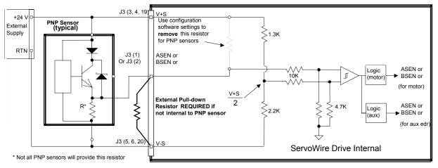
Figure 11, Schematic of ASEN and BSEN wiring for NPN and PNP sensors
