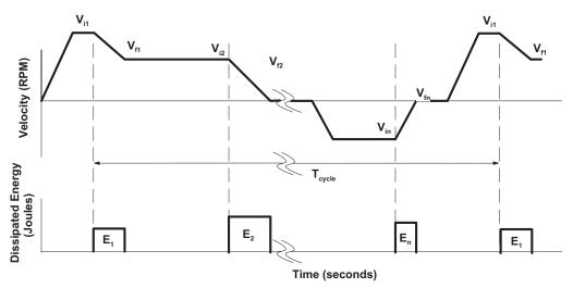
Figure 27, Regeneration during deceleration.
