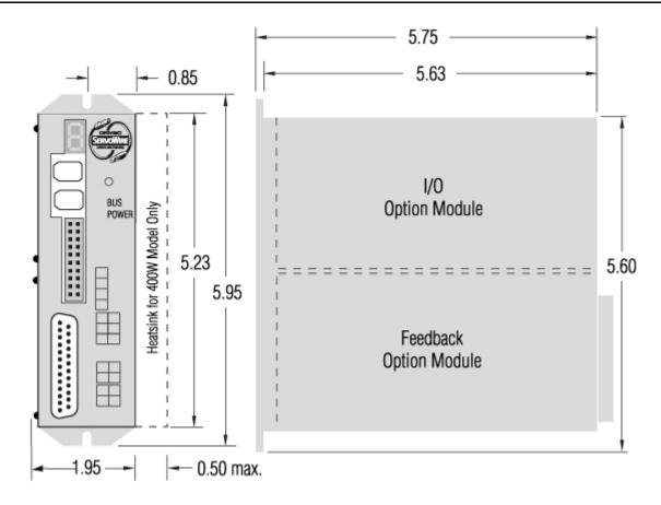
Figure 4, ServoWire SM Low Power Drives (24-96 VDC) Outline Drawing
