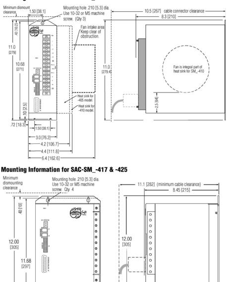
Figure 2, ServoWire SM Drives (460 VAC input) Outline Drawings (1 of 2)
