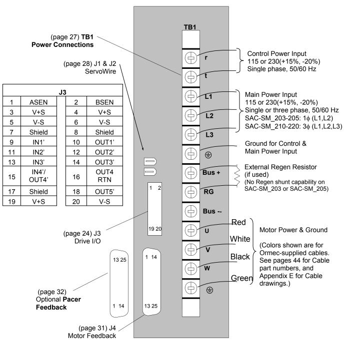
Figure 6, ServoWire SM Drive Connections Overview (SM\_203 – SM\_220)
