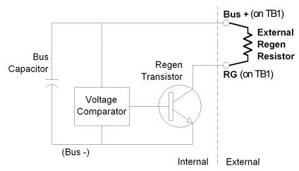
Figure 26, Simplified Schematic of Shunt Regulator
