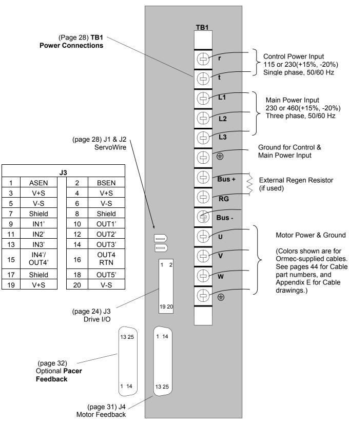
Figure 8, ServoWire SM Drive Connections Overview (SM\_405 - SM\_410)
