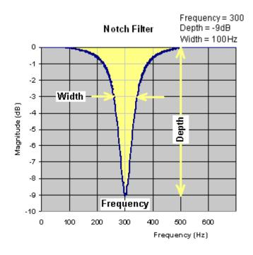
NOTCH FREQUENCY is the center frequency of the current loop's notch filter in Hertz. The center frequency of the notch measures the frequency at which the filter's magnitude reaches it's minimum value. Default = 300, range 1 to 2500.
