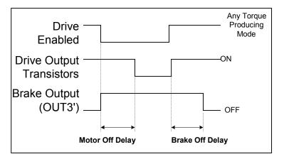
Figure 21, Brake Output Sequence of Operation
