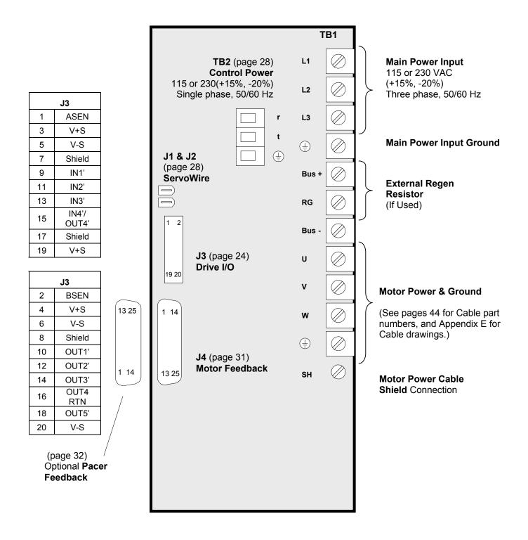
Figure 7, ServoWire SM Drive Connections Overview(SM\_225 – SM\_260)
