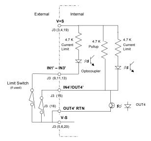
Figure 12, Schematic of IN1', IN2', IN3' and IN4'/OUT4' Inputs
