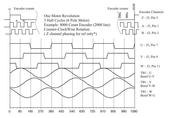
Figure 23, Hall signals and Motor Back EMF waveforms
