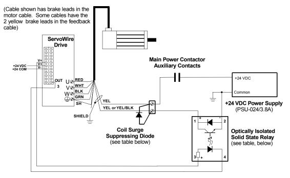
Figure 19, Fail-Safe Brake Interlock Circuit
