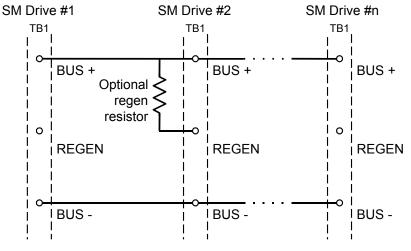
Figure 15, Bus Sharing Connections
